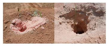
Figure 2 (L-R) Heavy ANFO after loading vs.  $\Delta E$  after loading
